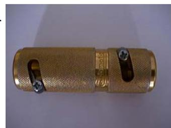
(<http://www.ripley-tools.com>). The "First Cut" end cuts the coax outer jacket, shield, and core, but not the center conductor. The center conductor is cut to the exact length needed, 5/8".
