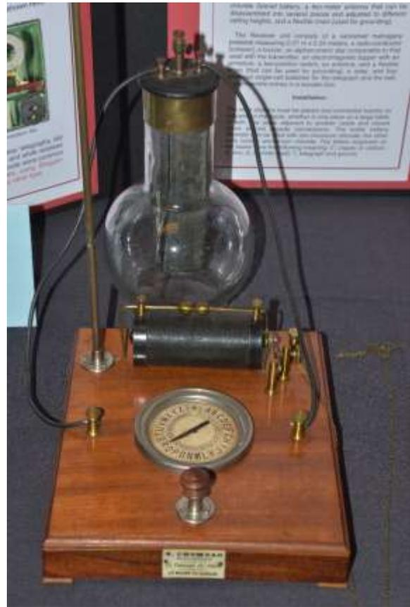
Figure 3. Spark transmitter for the demonstration telegraph. Receiver is in Fig 2.
