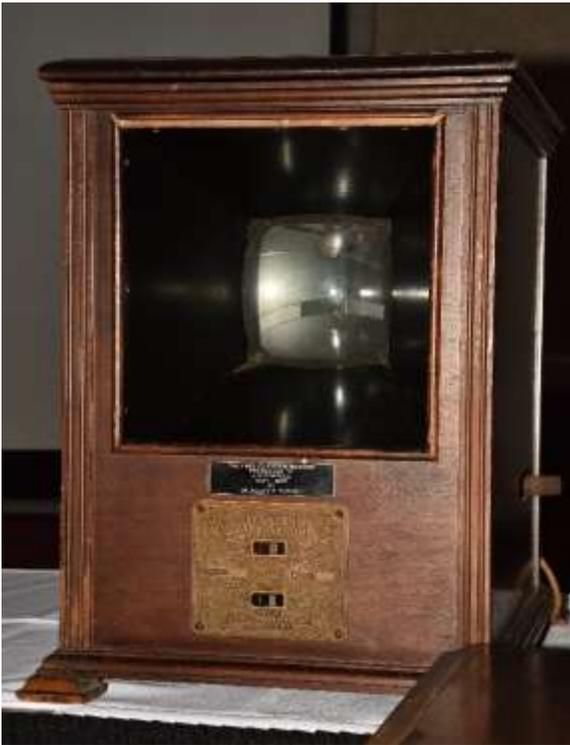
Fig 4. Jenkins Radiovisor originally presented to Jack Poppele by Allen Dumont in 1926. This is the television section. There is also the radio receiver and a horn speaker. This device uses a rotating drum and not a typical Nipkow disk.
