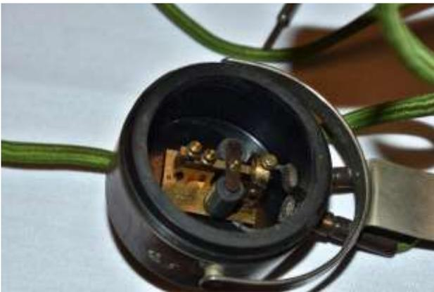
Fig. 1 Telegraph Earphone. Note tiny sounder in earphone.
