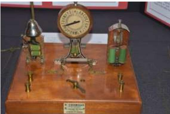
Fig 2. Receiver for demonstration wireless telegraph. This device used pulse modulation similar to an old telephone to determine the letter.
