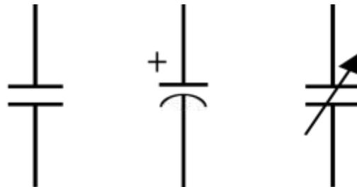
Fixed capacitor    Polarized capacitor    Variable capacitor
