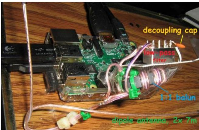
Joe says, "The antenna is just a dipole taped up to the walls of my living room and hallway." As you can see he made the balun and dipole from 24 ga speaker wire.
